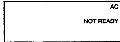
TYPICAL DISPLAY INDICATING OPEN PROTECTION ZONE
